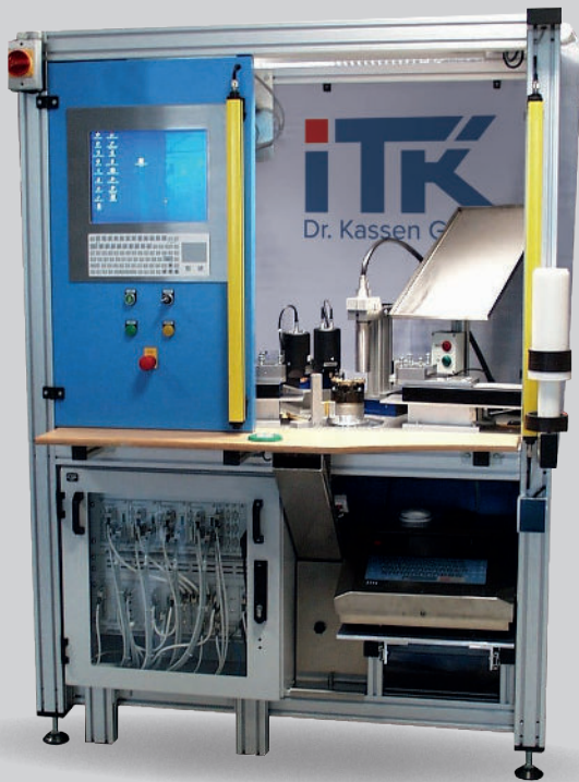
ABOVE: Rotary magnetization machine RIGHT: Writing system as part of the magnetization machine
