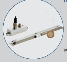
The integrated linear measuring system is based on magneto-resistive (MR) sensor technology and thus uses the special advantages of MR sensor technology such as freedom from maintenance, high dynamics, robustness and freedom from wear. In addition, the absolute measuring system makes time-consuming homing runs and end switches superfluous. The current position is known at all times.
